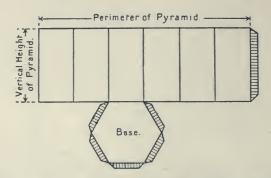
If sand is now used, it will be found that the pyramid is one third of the corresponding prism; *i.e.* its volume is  $\frac{1}{3}Ah$ , where A is the area of the base and h the vertical height.
